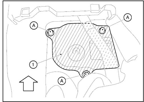
4. Remove the service plug using the following steps: (1) pull up and release the green lever, (2) press the locking tab to release and rotate fully upward (3) and pull the service plug completely out of its socket.
