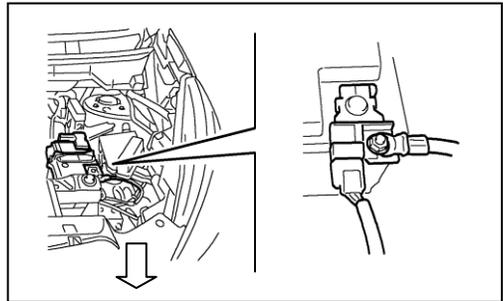
7. **Wait at least ten (10) minutes for complete discharge** of the high voltage capacitor after the power switch has been turned OFF.
