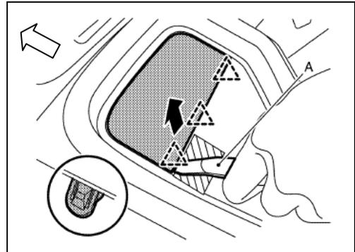
2. Remove the fixing screw (A) and disengage the metal fixing clips, and then remove the cover.
