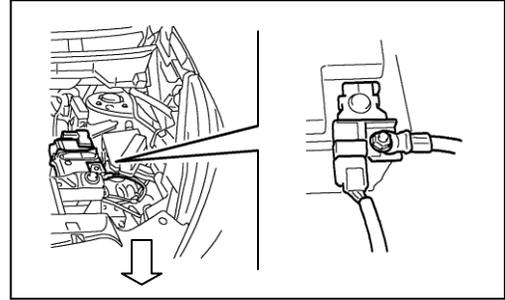
6. **Wait at least ten (10) minutes for complete discharge** of the high voltage capacitor after the fuses are pulled.
