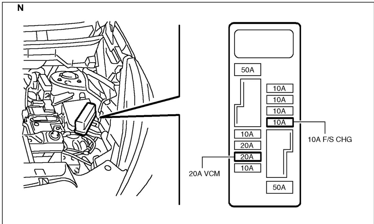
4. If you cannot identify the above fuses, remove all fuses in the fuse boxes.
