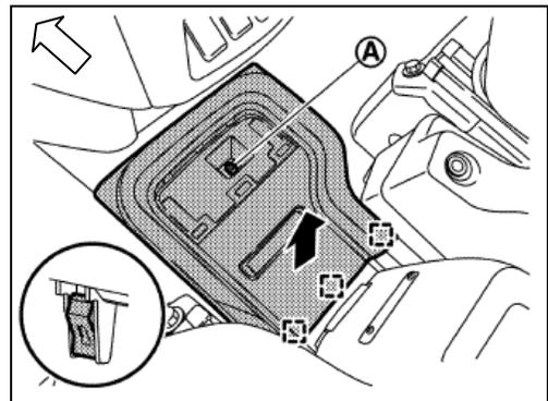
3. Remove the access cover bolts (A) and remove the cover (1)
