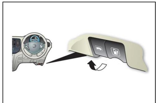
2. Press and expand the pawls on the sides of the fuse box and remove the fuse box (1) from its housing.
