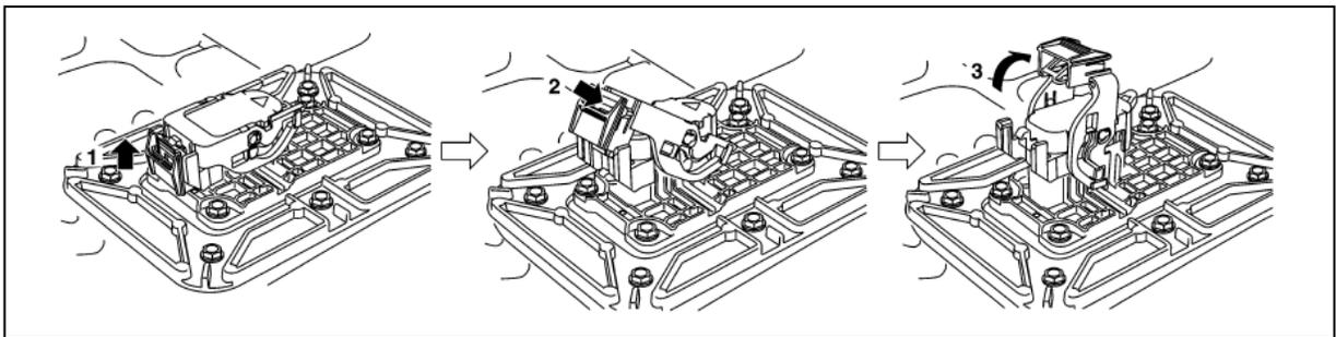
5. **Wait at least ten (10) minutes for complete discharge** of the high voltage capacitor after the service plug has been removed.
