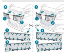
► For each very cold climate screen 1 and 2, cut the mounting tabs according to the type of grille A or B that is fitted to the vehicle.
