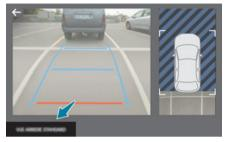
To activate the camera located on the tailgate, engage reverse gear and do not exceed a speed of 6 mph (10 km/h).
