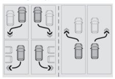
A manoeuvre selection page is displayed on the touch screen: by default, the "Entry" page if the vehicle has been running since the ignition was switched on, otherwise, the "Exit" page.
