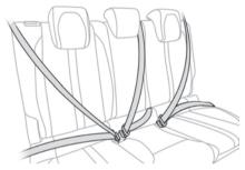
Each of the rear seats has a three-point seat belt with inertia reel.
