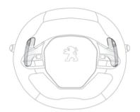
► Pull the "+" or "-" paddle towards you and release to shift up or down a gear, respectively.
