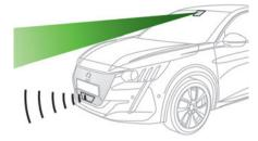
The vehicle has a multifunction camera located at the top of the windscreen and, depending on version, a radar located in the front bumper.
