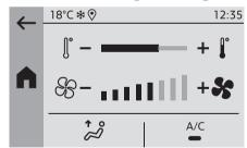
Depending on equipment/Depending on version. Manage various temperature and air flow settings.
