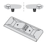
► Press the control to display the modes on the instrument panel, and depending on version, on the screen with PEUGEOT Connect Nav.
