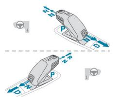
► Move the selector by pressing it forwards (N or R) or rearwards (N or D) once or twice, passing the point of resistance if necessary. The push selector returns to its initial position when released.
