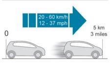
▶ Drive immediately for approximately 3 miles (5 kilometres) at reduced speed (between 12 and 37 mph (20 and 60 km/h)) to plug the puncture.
