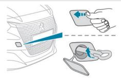
► Unclip the cover by pressing at its top lefthand corner
