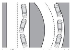
The system assesses the driver's level of alertness, fatigue and distraction by identifying trajectory changes in relation to the lane markings.
