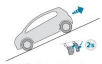
Facing downhill, with the vehicle stationary and reverse gear engaged, the vehicle is held for a short time when the driver releases the brake pedal.
