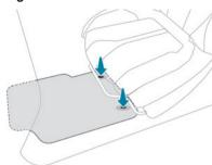
When fitting it on the driver's side, only use the mountings present on the carpet (a "click" indicates proper locking).
