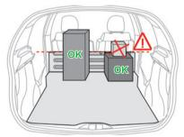
Do not place objects above the load retaining partition.
