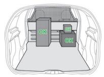
If the vehicle is equipped with a safety grille, objects can be placed above the load retaining partition.
