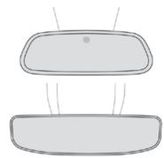
This system automatically and progressively transitions between day and night modes, using a sensor that measures the light entering from the rear of the vehicle.
