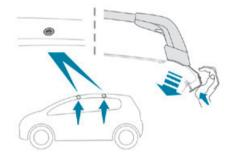
You must only attach the transverse bars to the four fixing points located on the roof frame. These points are concealed by the vehicle doors when the doors are closed.
