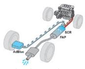
To respect the environment and ensure compliance with the Euro 6 standard, without adversely affecting the performance or fuel consumption of its Diesel engines, PEUGEOT has taken the decision to equip its vehicles with a system that associates SCR (Selective Catalytic Reduction) with a Diesel Particle Filter (DPF) for the treatment of exhaust gases.
