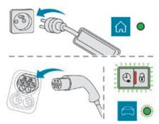
► Connect the charging cable from the control unit to the domestic socket.
