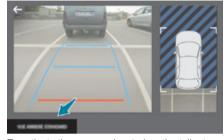
To activate the camera, located on the tailgate, engage reverse and keep the speed of the vehicle below 6 mph (10 km/h).
