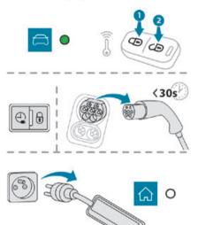
When charging is complete, the green **CHARGE** indicator lamp on the control unit comes on fixed.
