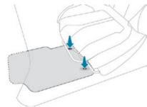
When fitting the mat for the first time, on the driver's side use only the fasteners supplied in the enclosed sachet
