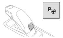
► Press the button on the gear selector or, on the touch screen, select **Driving** / **Vehicle** > **Full Park Assist**.
