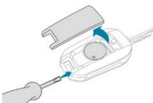
With Keyless Entry and Starting Battery type: CR2032 / 3 volts.
