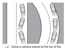
windscreen, the system assesses the driver's level of vigilance, fatigue or distraction by identifying variations in trajectory compared to the lane markings.
